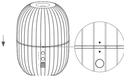
3. Replace the cover. Make sure the cover marking dot aligns with the base marking dot.
