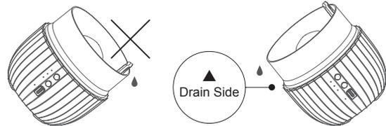
2. Pour all the remaining water out from the drain side.
